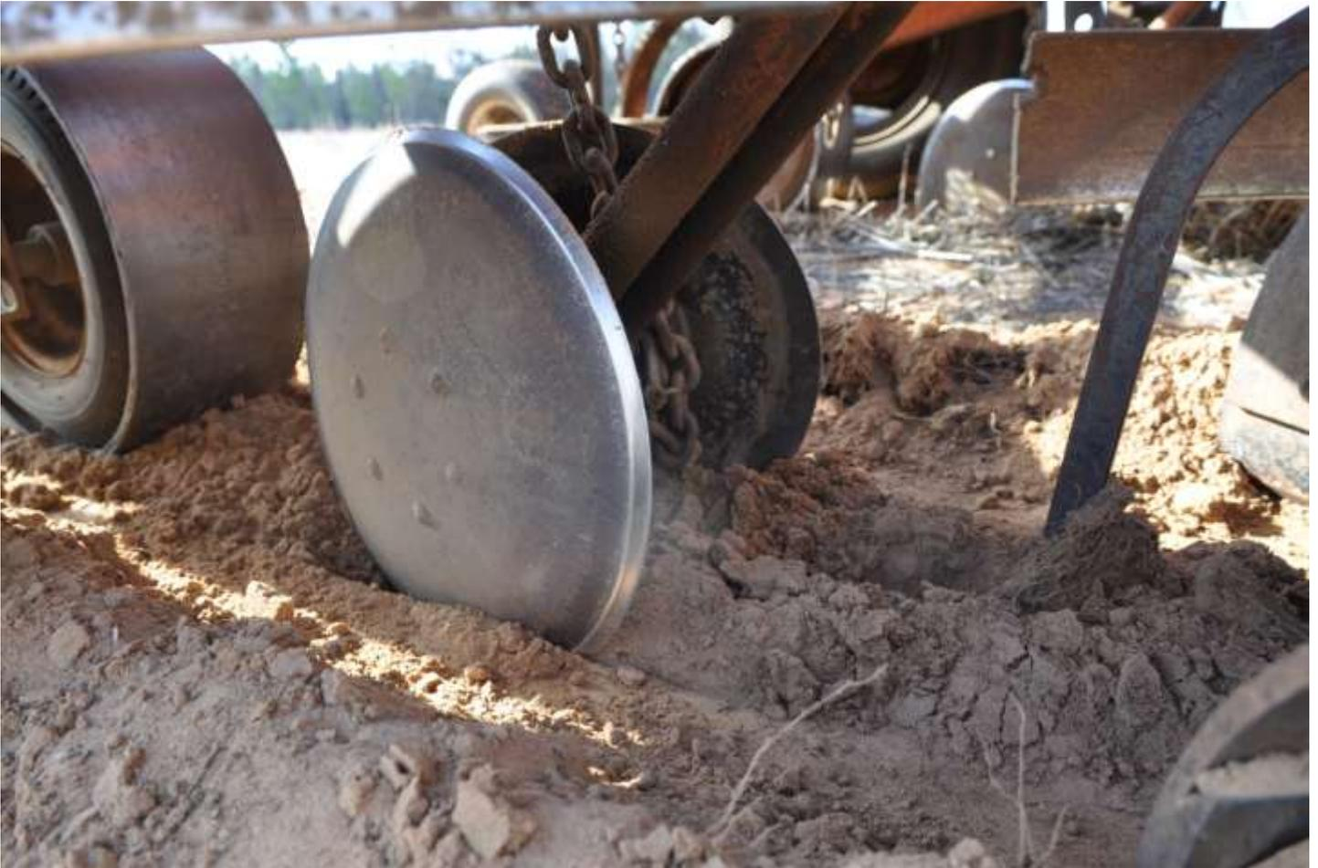
Figure 2. Soil preparation achieved with the CommVeg precision seeder. The machine was travelling from left to right and the image shows the view behind the scalper, showing the ripper (spring tyne), small tillage disks and the floating seeder arm which places the seed
