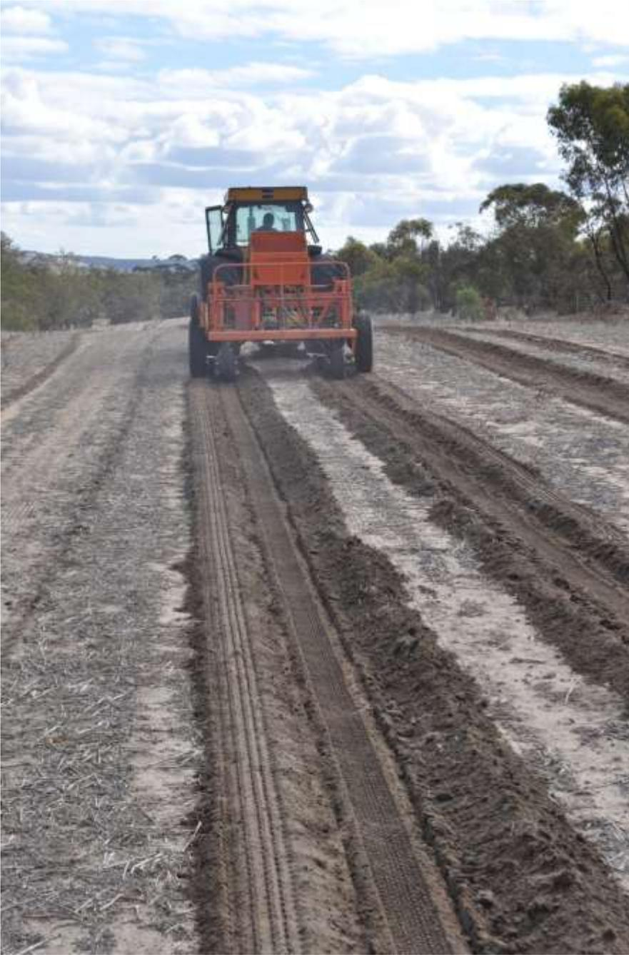
Figure 1 Seeding with a precision seeder designed by Geoff Woodall (CommVeg seeder). As shown in this image, good weed control, precision sowing, and a stable soil environment are key to successful direct seeding.
